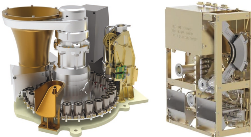
Figure 1 Rendering of the ProSPA payload with the Sample Inlet System (left) and Sample Analysis Suite (right). Credit: ESA.
